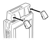
• To remove the screw covers, insert a flat blade screwdriver at the locations indicated by arrows in the illustration.
